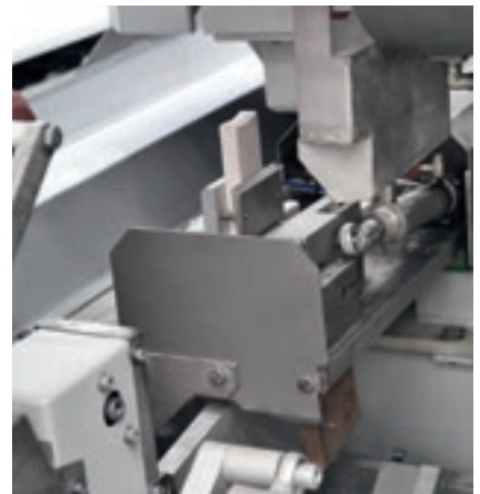
Three-position stick dresser for profiling and shaping diamond wheels.
