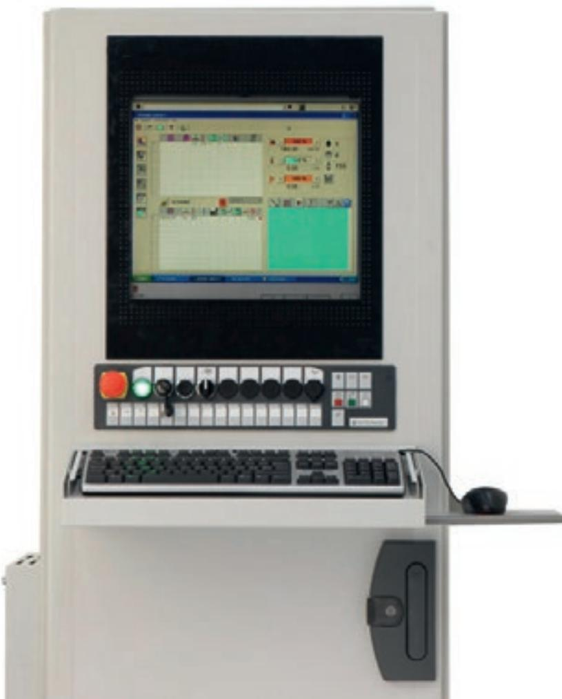
The operator interface is simple and intuitive, and enables cutting programmes generated by a range of the optimisers present on the market to be imported, courtesy of the integrated OTD (Optimiser Transferring Data) universal interface that automatically defines cutting parameters and generates the programme for the cutting table.
