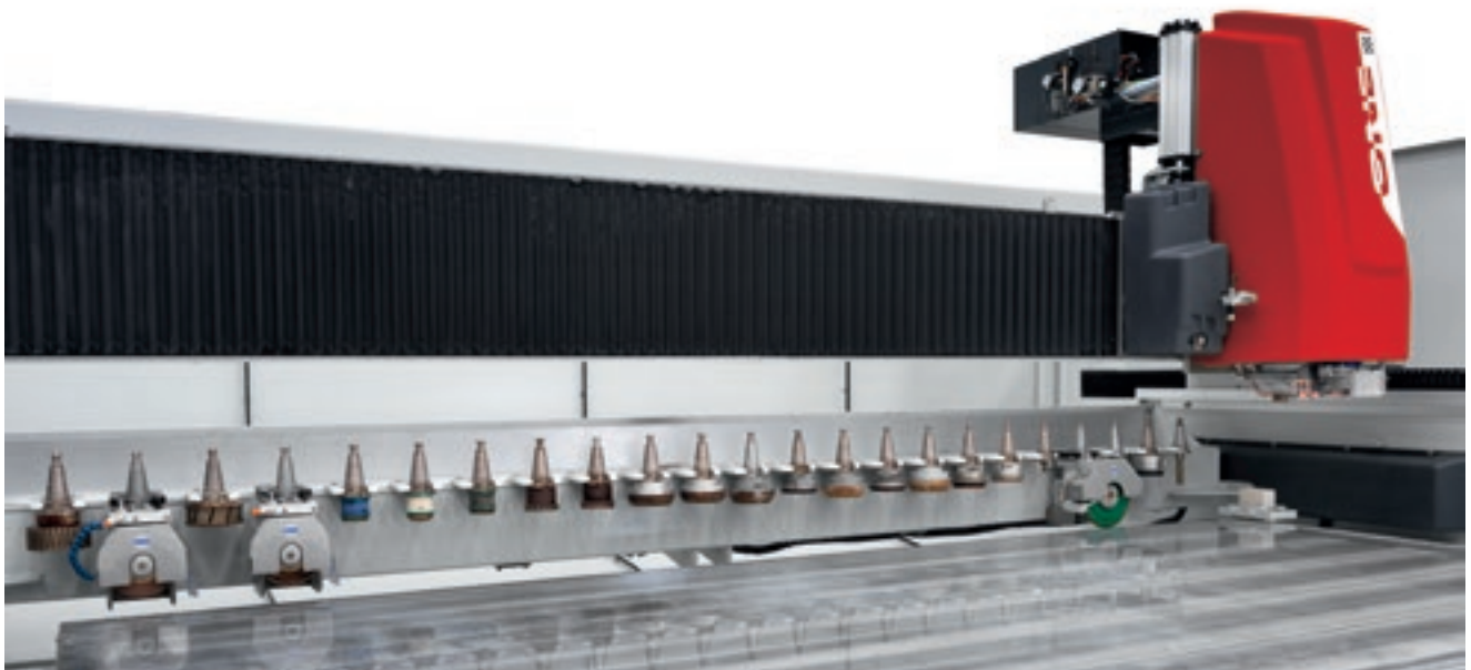
Rear tool magazine with 23 positions.
