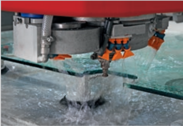
Complete machining of a door: milling and notch grinding, grinding and peripheral polishing.
