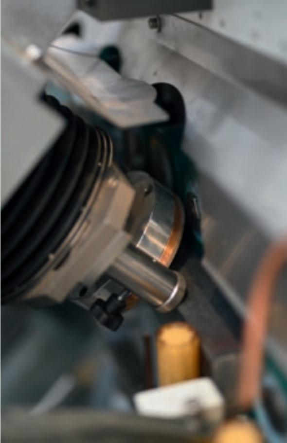
Creation of chamfers of a consistent size courtesy of the upper chamfering unit which "adapts" to the thickness of the material, with an automatic and manual slide block system.
