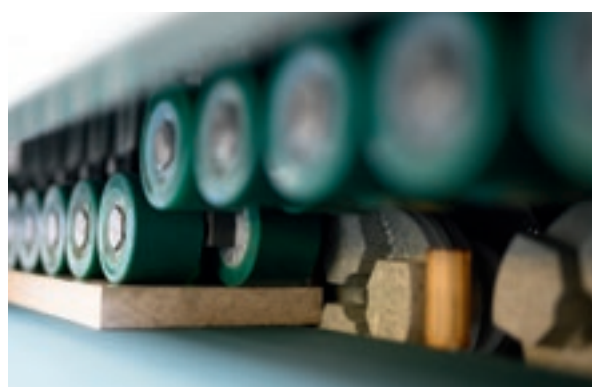
Duplex presser wheels for a minimum head width of 120 mm.
