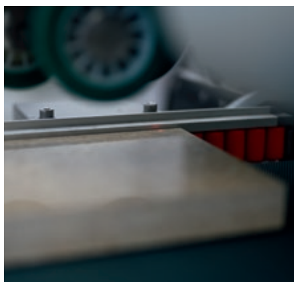
Automatic reading of the thickness of the panel for automatic adjustment of the devices.
