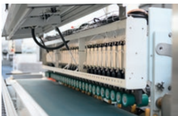
Pneumatic pressers as standard for machining panels of different thicknesses at the same time, ensuring uniform pressure which is essential when processing ceramic materials, especially those that are thin.
